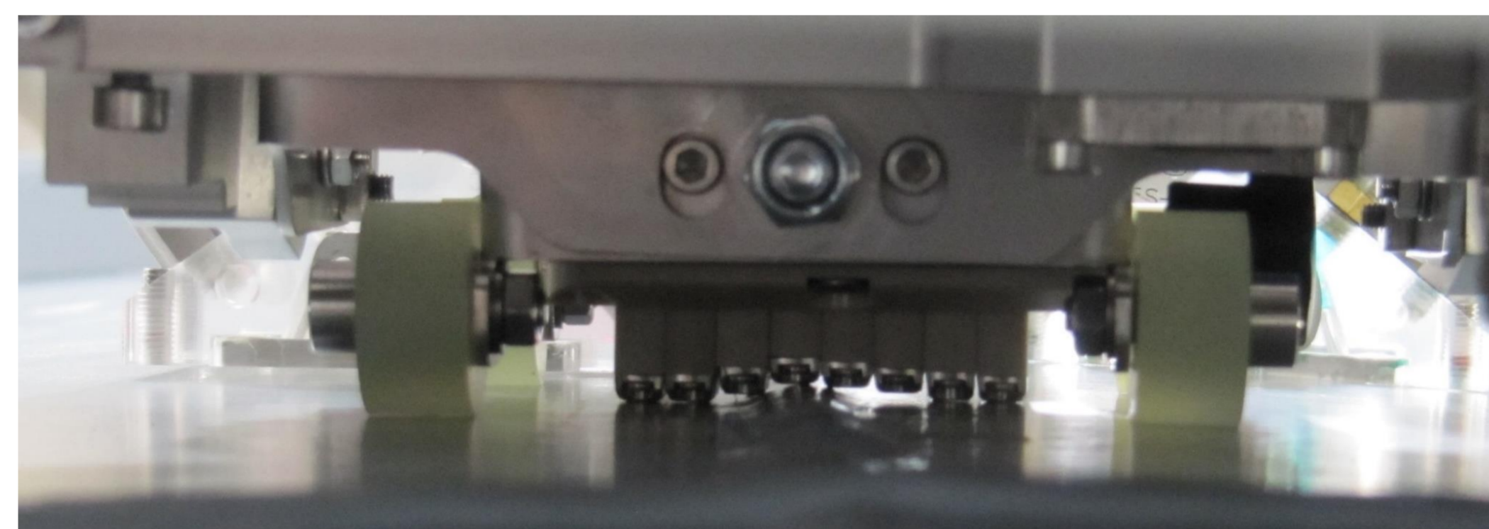
ACFM array probe on in the robot
