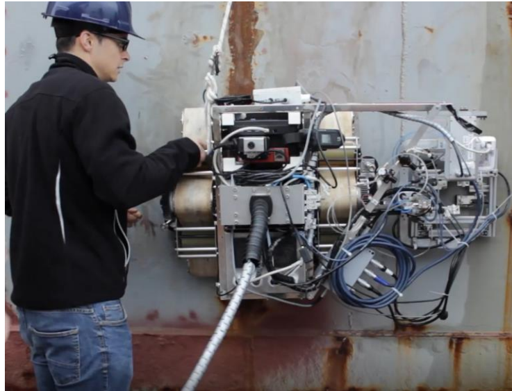
The old X-Scan with sensors outside the main structure
